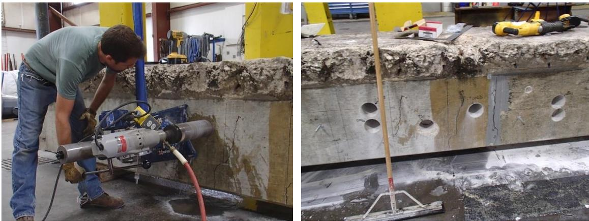
Figure 92—Coring of bridge girders
