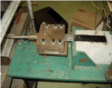
Figure 24—Direct shear test setup (Lai et al., 2009)
