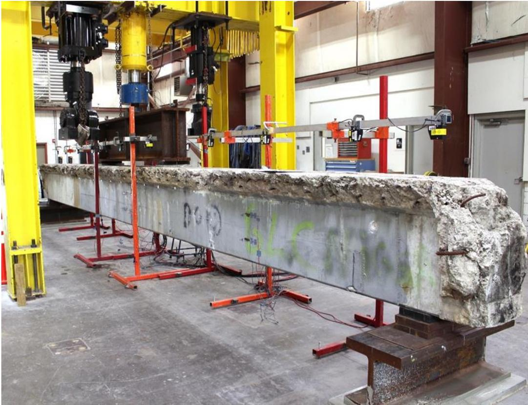
Figure 110—Girder loaded in test frame
