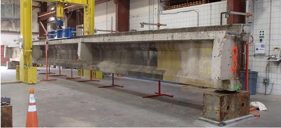
Figure 238—Girder loaded in test frame
