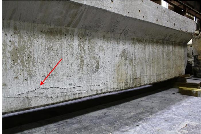
Figure 143—Horizontal crack on Girder 3-1 indicated by red arrow
