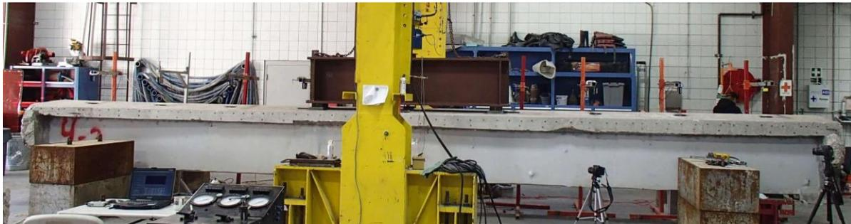
Figure 167—Girder loaded in test frame
