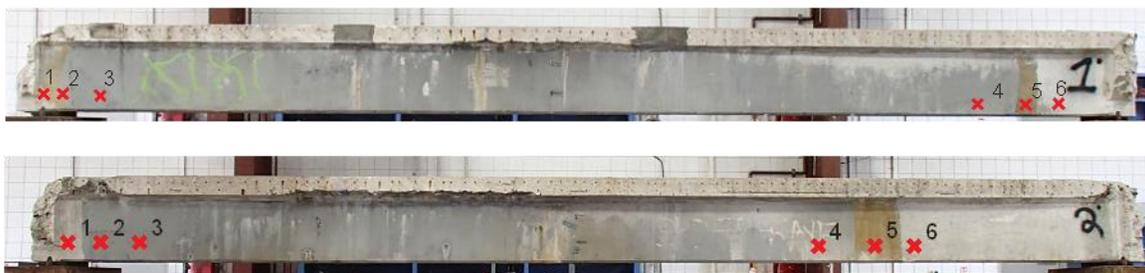
Figure 93—Approximate coring locations for Cl<sup>-</sup> penetration profile cores on each girder
