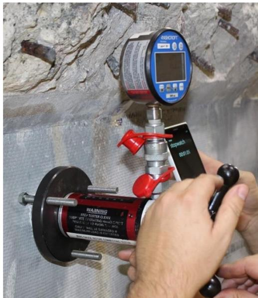
Figure 101—Direct pull-off test setup
